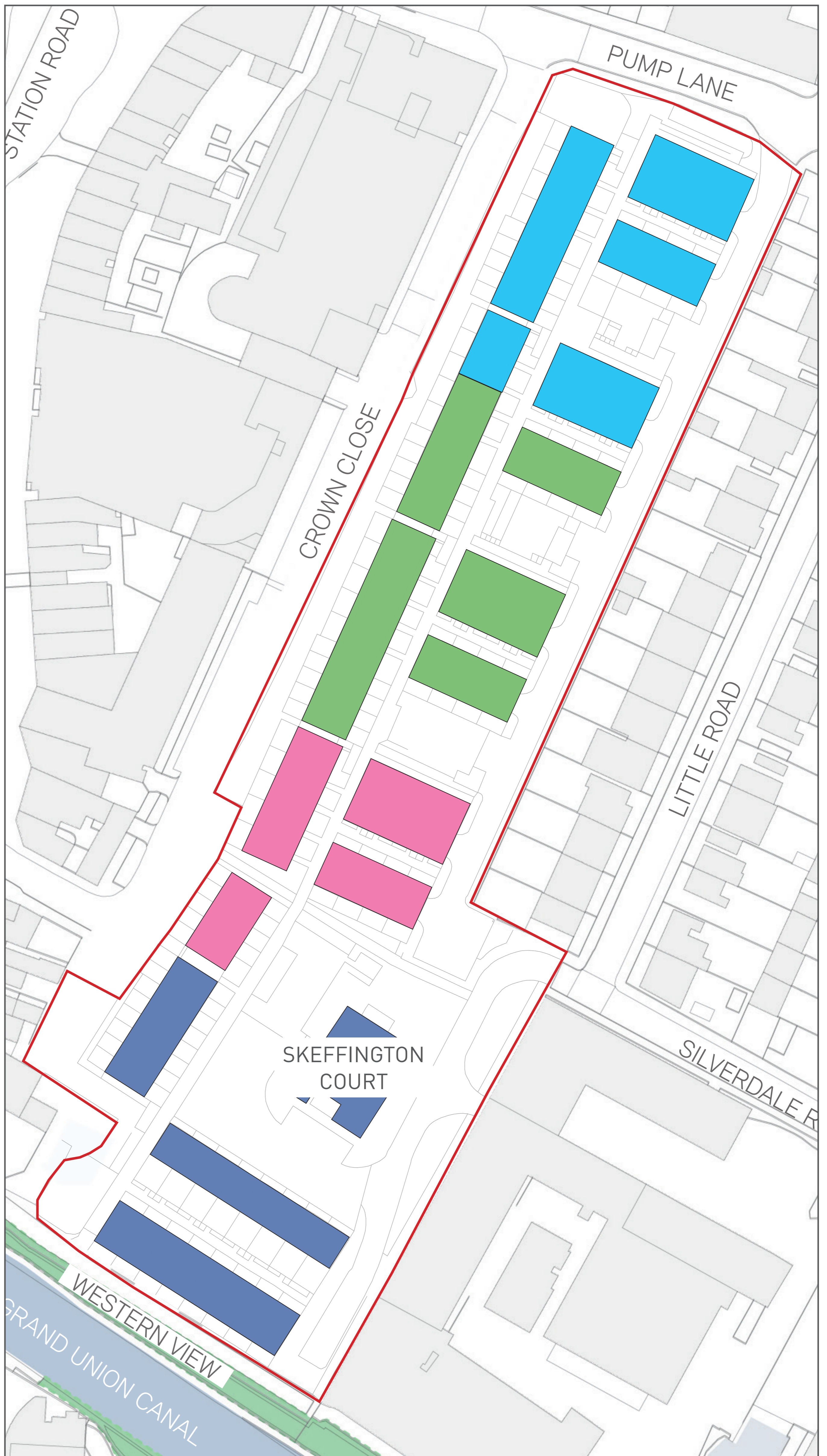
Indicative demolition phasing
