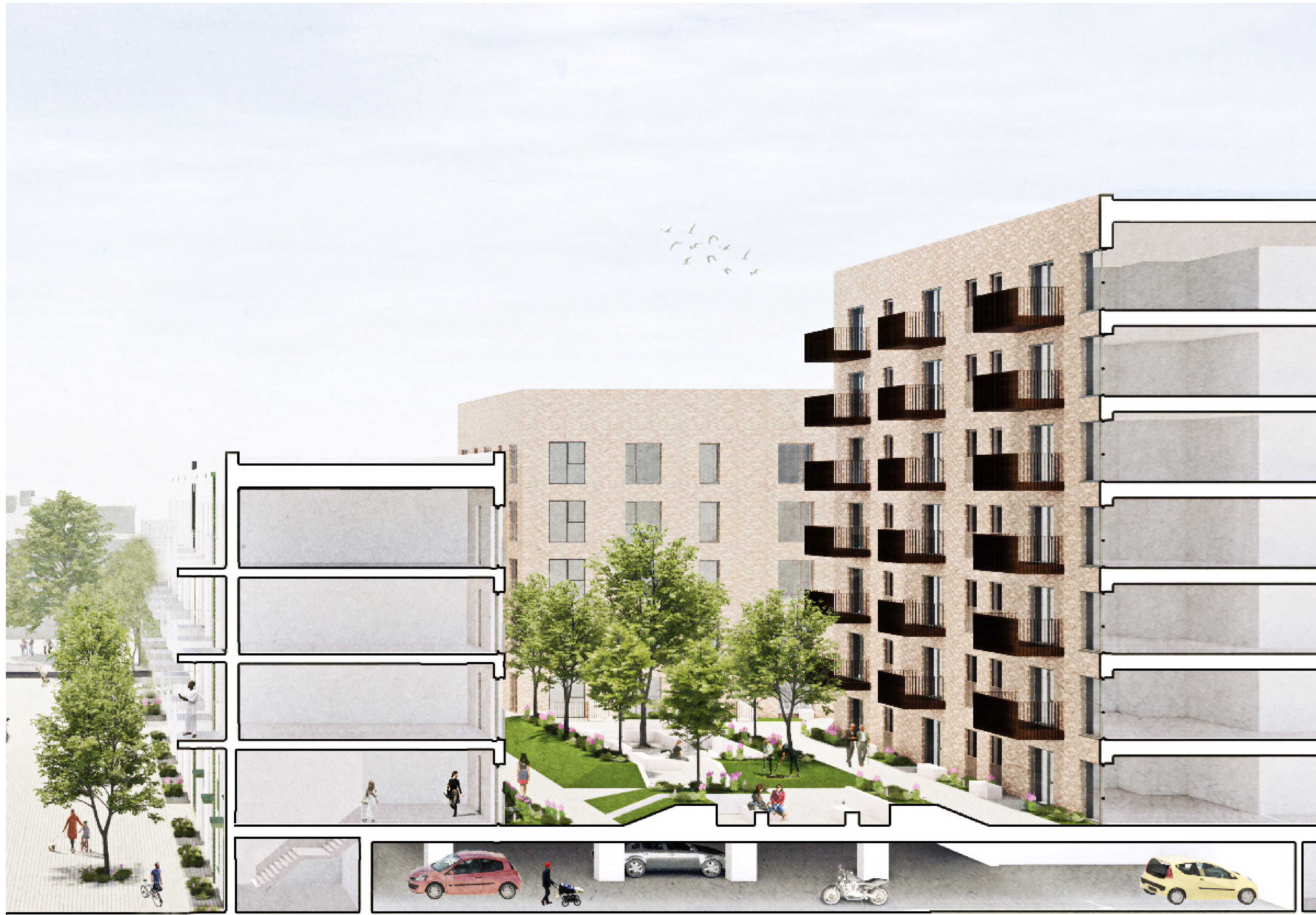
A cut through sketch showing the first floor resident only courtyard with parking below
